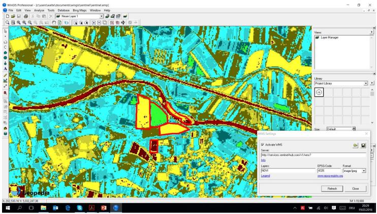
Sentinel NDVI image as WMS service within WinGIS professional and as service sent via JPEG to smartphones and via bluetooth to machine hardware as fundament for PF
